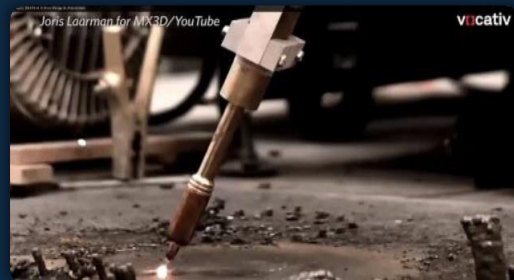
MX3D Bridge Printing
